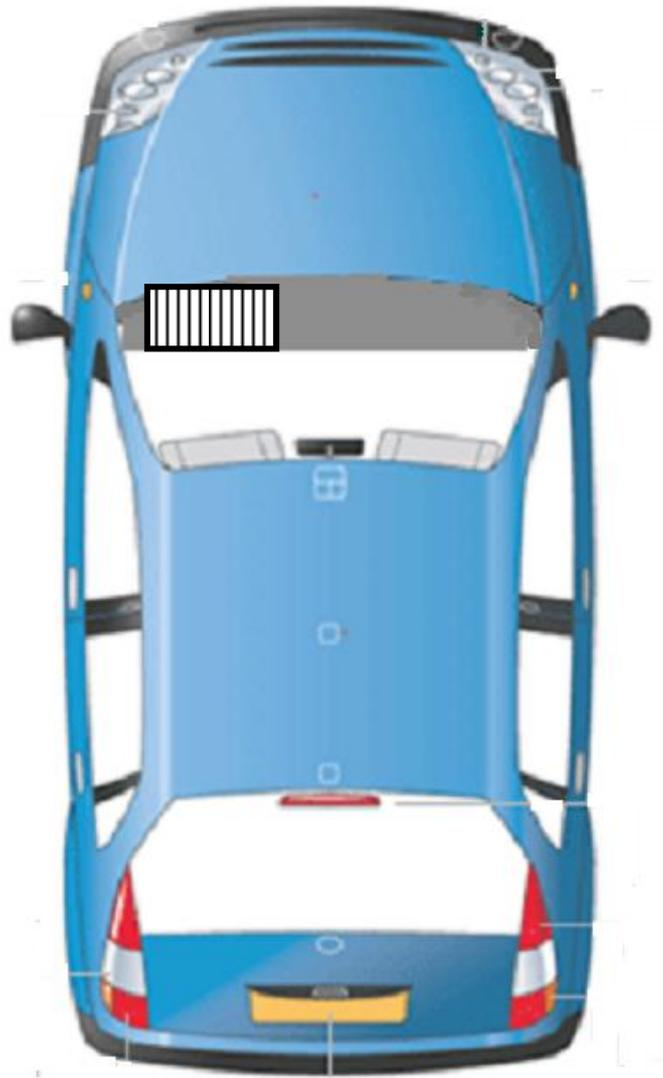
1. The cabin filter is located between the glove box and the passenger footwell.
