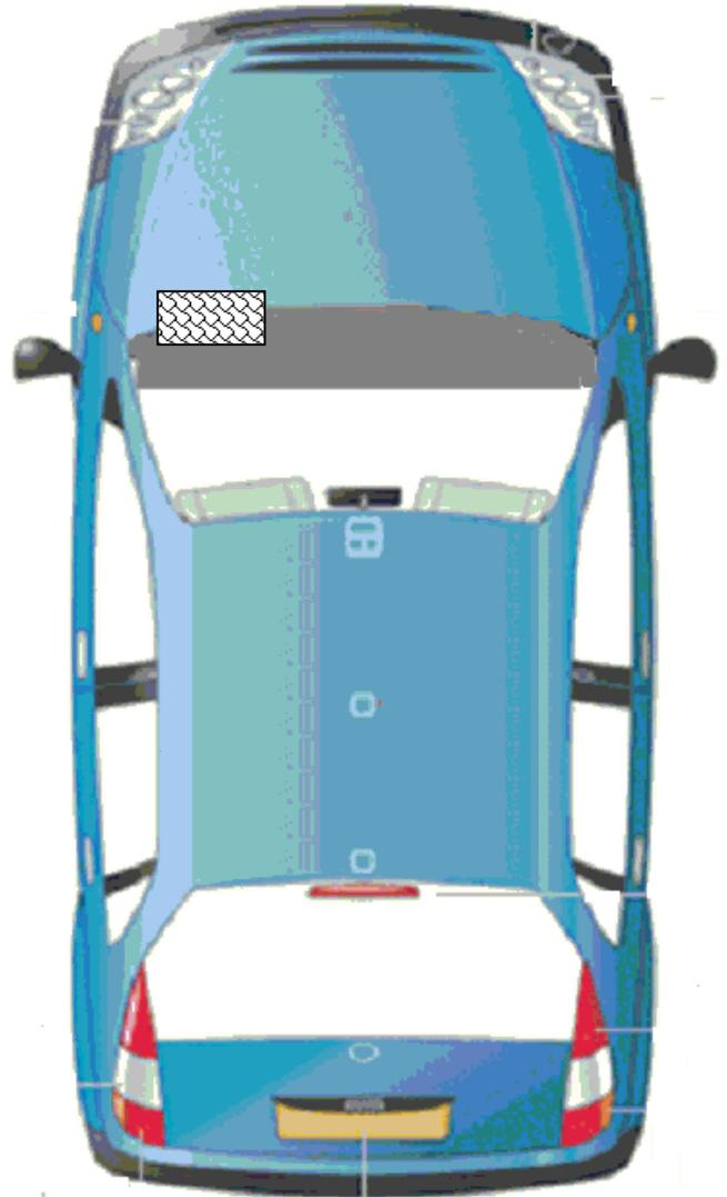
1. The Cabin Filter can be found in the engine compartment at the base of the windscreen.
