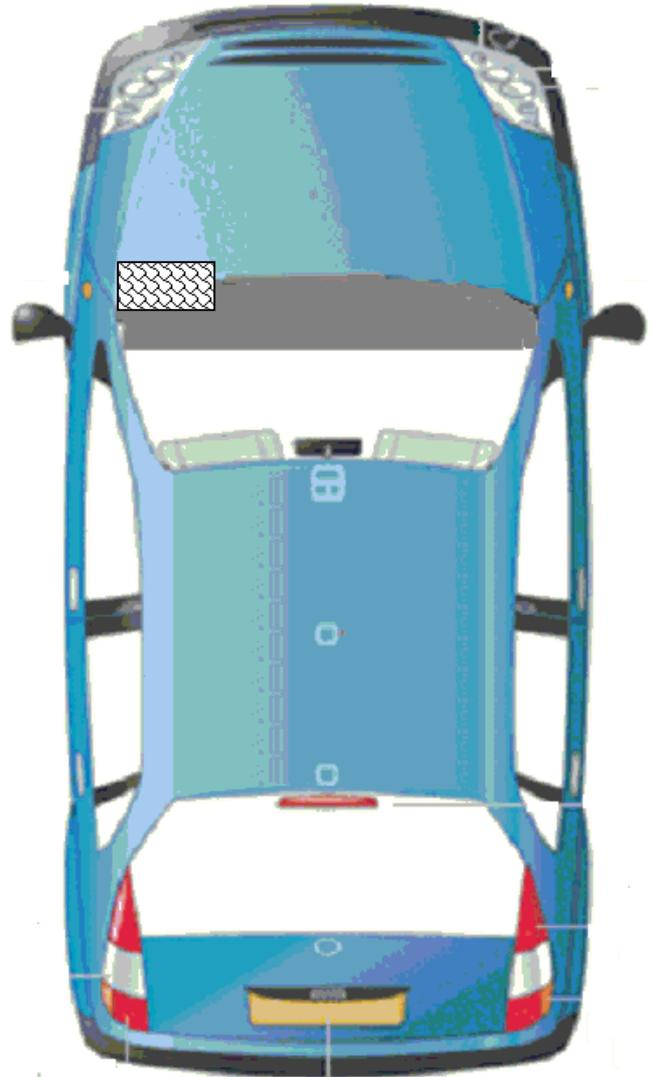
1. The cabin filter can be found on the passenger side under the bonnet at the base of the windscreen.
